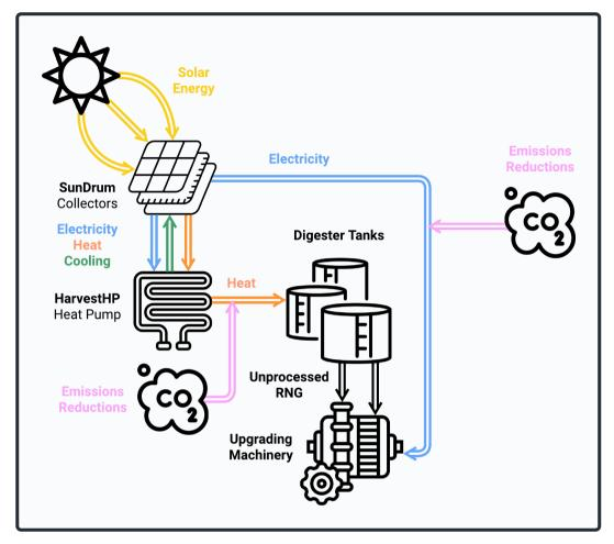
SunDrum Solar captures heat and electricity with an integrated heat pump to provide 24/7 heating for anaerobic digestion systems. The power drawn by the heat pump is provided by the panel, and a SunDrum system reduces - and in many cases eliminates - the need for expensive battery and thermal storage.
