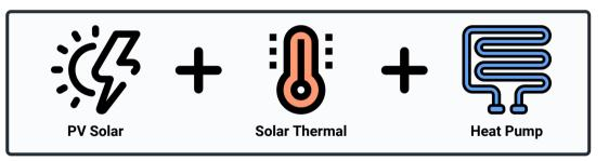
SunDrum Collectors mount directly behind conventional photovoltaic (PV) panels. A heat transfer fluid (propylene glycol) moves heat from the panels to an integrated heat pump to provide water heating.
